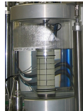
Photo 9.1 Triaxial compression test
